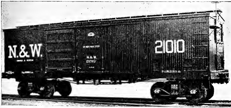
Fig. 5. FRUIT CAR. NORFOLK & WESTERN RAILROAD. Length, 34 ft. 8 ins. Capacity, 65,000 lbs. Weight, 31,500 lbs. Grated Doors and Ventilators. Equipped with Rigid Diamond Trucks.
